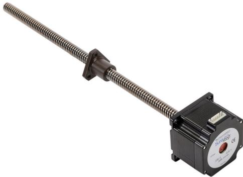
SureStep stepper motor linear actuator, external nut, NEMA 23 frame, IP40, single stack, 2.1A, 12in lead screw length, 6mm/rev, 12mm lead screw diameter, screw code H, no end machining.
