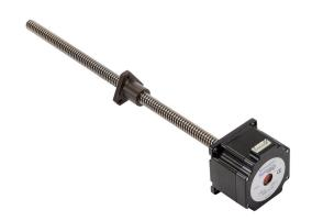
SureStep stepper motor linear actuator, external nut, NEMA 23 frame, IP40, single stack, 2.1A, 12in lead screw length, 6mm/rev, 12mm lead screw diameter, screw code H, no end machining.
