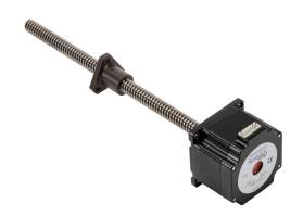
SureStep stepper motor linear actuator, external nut, NEMA 23 frame, IP40, single stack, 2.1A, 9in lead screw length, 6mm/rev, 12mm lead screw diameter, screw code H, no end machining.
