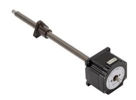
SureStep stepper motor linear actuator, external nut, encoder ready, NEMA 23 frame, IP40, single stack, 2.1A, 9in lead screw length, 6mm/rev, 12mm lead screw diameter, screw code H, journal and groove end machining.
