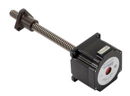
SureStep stepper motor linear actuator, external nut, NEMA 23 frame, IP40, single stack, 2.1A, 6in lead screw length, 6mm/rev, 12mm lead screw diameter, screw code H, no end machining.
