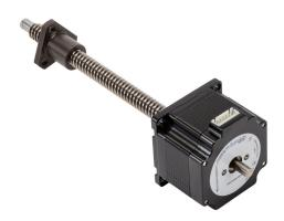
SureStep stepper motor linear actuator, external nut, encoder ready, NEMA 23 frame, IP40, single stack, 2.1A, 6in lead screw length, 6mm/rev, 12mm lead screw diameter, screw code H, journal and groove end machining.
