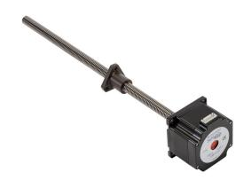
SureStep stepper motor linear actuator, external nut, NEMA 23 frame, IP40, single stack, 2.1A, 12in lead screw length, 2mm/rev, 12mm lead screw diameter, screw code G, no end machining.
