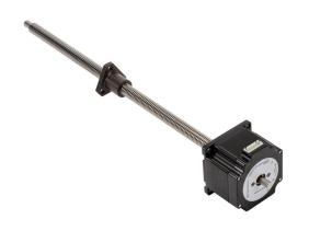
SureStep stepper motor linear actuator, external nut, encoder ready, NEMA 23 frame, IP40, single stack, 2.1A, 12in lead screw length, 2mm/rev, 12mm lead screw diameter, screw code G, journal and groove end machining.
