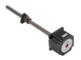
SureStep stepper motor linear actuator, external nut, NEMA 23 frame, IP40, single stack, 2.1A, 9in lead screw length, 2mm/rev, 12mm lead screw diameter, screw code G, no end machining.
