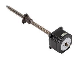
SureStep stepper motor linear actuator, external nut, encoder ready, NEMA 23 frame, IP40, single stack, 2.1A, 9in lead screw length, 2mm/rev, 12mm lead screw diameter, screw code G, journal and groove end machining.
