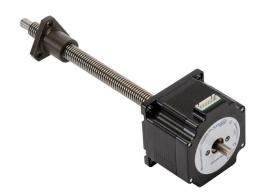
SureStep stepper motor linear actuator, external nut, encoder ready, NEMA 23 frame, IP40, single stack, 2.1A, 6in lead screw length, 2mm/rev, 12mm lead screw diameter, screw code G, journal and groove end machining.
