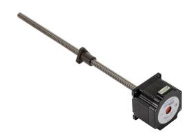
SureStep stepper motor linear actuator, external nut, NEMA 23 frame, IP40, single stack, 2.1A, 12in lead screw length, 10.5mm/rev, 10mm lead screw diameter, screw code F, no end machining.
