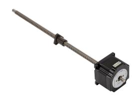
SureStep stepper motor linear actuator, external nut, encoder ready, NEMA 23 frame, IP40, single stack, 2.1A, 12in lead screw length, 10.5mm/rev, 10mm lead screw diameter, screw code F, journal and groove end machining.
