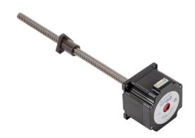
SureStep stepper motor linear actuator, external nut, NEMA 23 frame, IP40, single stack, 2.1A, 9in lead screw length, 10.5mm/rev, 10mm lead screw diameter, screw code F, no end machining.
