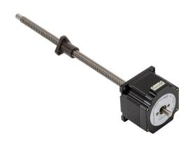
SureStep stepper motor linear actuator, external nut, encoder ready, NEMA 23 frame, IP40, single stack, 2.1A, 9in lead screw length, 10.5mm/rev, 10mm lead screw diameter, screw code F, journal and groove end machining.
