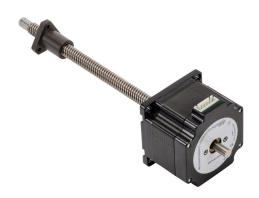
SureStep stepper motor linear actuator, external nut, encoder ready, NEMA 23 frame, IP40, single stack, 2.1A, 6in lead screw length, 10.5mm/rev, 10mm lead screw diameter, screw code F, journal and groove end machining.
