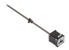
SureStep stepper motor linear actuator, external nut, encoder ready, NEMA 17 frame, IP40, triple stack, 2A, 12in lead screw length, 8mm/rev, 8mm lead screw diameter, screw code E, journal and groove end machining.
