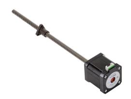
SureStep stepper motor linear actuator, external nut, NEMA 17 frame, IP40, triple stack, 2A, 9in lead screw length, 8mm/rev, 8mm lead screw diameter, screw code E, no end machining.
