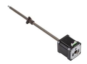
SureStep stepper motor linear actuator, external nut, encoder ready, NEMA 17 frame, IP40, triple stack, 2A, 9in lead screw length, 8mm/rev, 8mm lead screw diameter, screw code E, journal and groove end machining.
