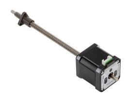
SureStep stepper motor linear actuator, external nut, encoder ready, NEMA 17 frame, IP40, triple stack, 2A, 6in lead screw length, 8mm/rev, 8mm lead screw diameter, screw code E, journal and groove end machining.
