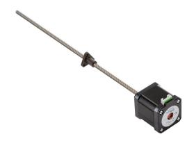
SureStep stepper motor linear actuator, external nut, NEMA 17 frame, IP40, triple stack, 2A, 12in lead screw length, 0.5in/rev, 0.25in lead screw diameter, screw code B, no end machining.
