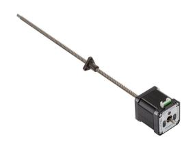
SureStep stepper motor linear actuator, external nut, encoder ready, NEMA 17 frame, IP40, triple stack, 2A, 12in lead screw length, 0.5in/rev, 0.25in lead screw diameter, screw code B, journal and groove end machining.
