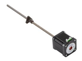
SureStep stepper motor linear actuator, external nut, NEMA 17 frame, IP40, triple stack, 2A, 9in lead screw length, 0.5in/rev, 0.25in lead screw diameter, screw code B, no end machining.
