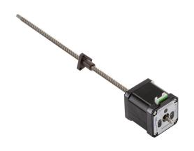
SureStep stepper motor linear actuator, external nut, encoder ready, NEMA 17 frame, IP40, triple stack, 2A, 9in lead screw length, 0.5in/rev, 0.25in lead screw diameter, screw code B, journal and groove end machining.
