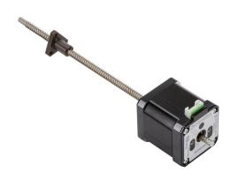
SureStep stepper motor linear actuator, external nut, encoder ready, NEMA 17 frame, IP40, triple stack, 2A, 6in lead screw length, 0.5in/rev, 0.25in lead screw diameter, screw code B, journal and groove end machining.
