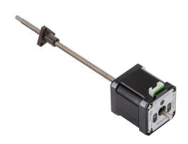
SureStep stepper motor linear actuator, external nut, encoder ready, NEMA 17 frame, IP40, triple stack, 2A, 6in lead screw length, 0.5in/rev, 0.25in lead screw diameter, screw code B, journal and groove end machining.
