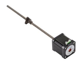
SureStep stepper motor linear actuator, external nut, NEMA 17 frame, IP40, triple stack, 2A, 9in lead screw length, 0.25in/rev, 0.25in lead screw diameter, screw code A, no end machining.
