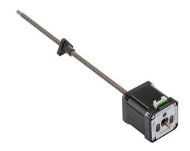
SureStep stepper motor linear actuator, external nut, encoder ready, NEMA 17 frame, IP40, triple stack, 2A, 9in lead screw length, 0.25in/rev, 0.25in lead screw diameter, screw code A, journal and groove end machining.
