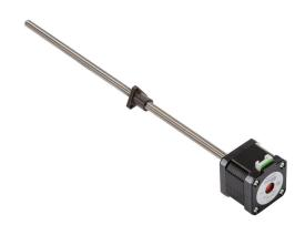
SureStep stepper motor linear actuator, external nut, NEMA 17 frame, IP40, double stack, 2A, 12in lead screw length, 1.25mm/rev, 8mm lead screw diameter, screw code D, no end machining.
