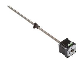
SureStep stepper motor linear actuator, external nut, encoder ready, NEMA 17 frame, IP40, double stack, 2A, 12in lead screw length, 1.25mm/rev, 8mm lead screw diameter, screw code D, journal and groove end machining.
