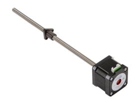
SureStep stepper motor linear actuator, external nut, NEMA 17 frame, IP40, double stack, 2A, 9in lead screw length, 1.25mm/rev, 8mm lead screw diameter, screw code D, no end machining.
