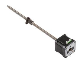
SureStep stepper motor linear actuator, external nut, encoder ready, NEMA 17 frame, IP40, double stack, 2A, 9in lead screw length, 1.25mm/rev, 8mm lead screw diameter, screw code D, journal and groove end machining.
