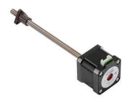
SureStep stepper motor linear actuator, external nut, NEMA 17 frame, IP40, double stack, 2A, 6in lead screw length, 1.25mm/rev, 8mm lead screw diameter, screw code D, no end machining.
