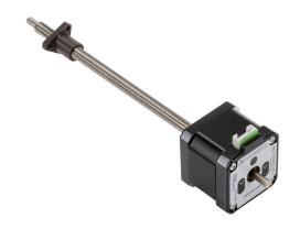
SureStep stepper motor linear actuator, external nut, encoder ready, NEMA 17 frame, IP40, double stack, 2A, 6in lead screw length, 1.25mm/rev, 8mm lead screw diameter, screw code D, journal and groove end machining.
