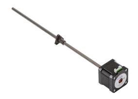
SureStep stepper motor linear actuator, external nut, NEMA 17 frame, IP40, double stack, 2A, 12in lead screw length, 3mm/rev, 6.5mm lead screw diameter, screw code C, no end machining.
