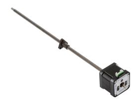
SureStep stepper motor linear actuator, external nut, encoder ready, NEMA 17 frame, IP40, double stack, 2A, 12in lead screw length, 3mm/rev, 6.5mm lead screw diameter, screw code C, journal and groove end machining.
