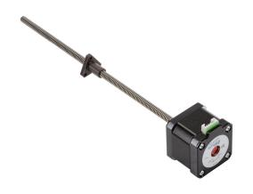
SureStep stepper motor linear actuator, external nut, NEMA 17 frame, IP40, double stack, 2A, 9in lead screw length, 3mm/rev, 6.5mm lead screw diameter, screw code C, no end machining.
