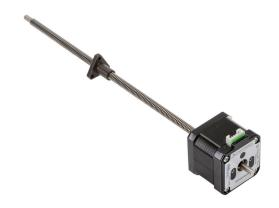
SureStep stepper motor linear actuator, external nut, encoder ready, NEMA 17 frame, IP40, double stack, 2A, 9in lead screw length, 3mm/rev, 6.5mm lead screw diameter, screw code C, journal and groove end machining.
