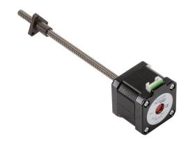
SureStep stepper motor linear actuator, external nut, NEMA 17 frame, IP40, double stack, 2A, 6in lead screw length, 3mm/rev, 6.5mm lead screw diameter, screw code C, no end machining.
