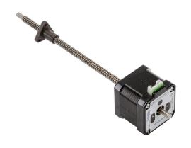
SureStep stepper motor linear actuator, external nut, encoder ready, NEMA 17 frame, IP40, double stack, 2A, 6in lead screw length, 3mm/rev, 6.5mm lead screw diameter, screw code C, journal and groove end machining.
