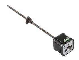
SureStep stepper motor linear actuator, external nut, encoder ready, NEMA 17 frame, IP40, double stack, 2A, 9in lead screw length, 0.25in/rev, 0.25in lead screw diameter, screw code A, journal and groove end machining.
