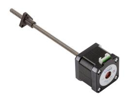
SureStep stepper motor linear actuator, external nut, NEMA 17 frame, IP40, double stack, 2A, 6in lead screw length, 0.25in/rev, 0.25in lead screw diameter, screw code A, no end machining.
