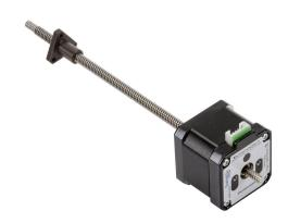
SureStep stepper motor linear actuator, external nut, encoder ready, NEMA 17 frame, IP40, double stack, 2A, 6in lead screw length, 0.25in/rev, 0.25in lead screw diameter, screw code A, journal and groove end machining.
