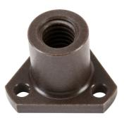
SureStep lead screw flange nut, replacement, triangular, 2mm/rev, 12mm lead screw diameter. For use with SureStep STP-LE series screw code G linear actuators.
