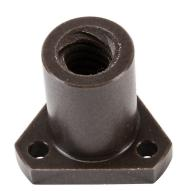
SureStep lead screw flange nut, replacement, triangular, 10.5mm/rev, 10mm lead screw diameter. For use with SureStep STP-LE series screw code F linear actuators.
