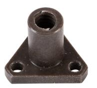
SureStep lead screw flange nut, replacement, triangular, 3mm/rev, 6.5mm lead screw diameter. For use with SureStep STP-LE series screw code C linear actuators.
