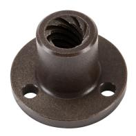
SureStep lead screw flange nut, round, 1in/rev, 0.5in lead screw diameter. For use with SureStep STP-LE series screw code K linear actuators.
