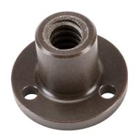
SureStep lead screw flange nut, round, 6mm/rev, 12mm lead screw diameter. For use with SureStep STP-LE series screw code H linear actuators.
