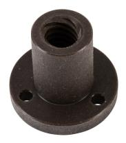
SureStep lead screw flange nut, round, 10.5mm/rev, 10mm lead screw diameter. For use with SureStep STP-LE series screw code F linear actuators.
