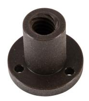
SureStep lead screw flange nut, round, 10.5mm/rev, 10mm lead screw diameter. For use with SureStep STP-LE series screw code F linear actuators.
