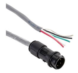
SureStep extension cable, 6-pin connector to pigtail, 6ft cable length. For use with SureStep MTRH series IP65 stepper motors.
