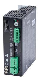
SureStep AC microstepping stepper drive, 2.5A per phase, 2-phase output, 90-240 VAC, bipolar, velocity and position mode, 200 to 25600 steps per revolution.
