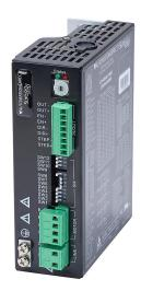
SureStep AC microstepping stepper drive, 2.5A per phase, 2-phase output, 90-240 VAC, bipolar, velocity and position mode, 200 to 25600 steps per revolution.
