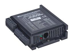
SureStep DC advanced microstepping stepper drive, 10A per phase, 2-phase output, 24-80 VDC, bipolar, velocity and position mode, 200 to 51200 steps per revolution, (1) RS-232 (RJ11) port(s).
